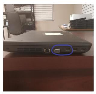
3. You will need to plug one end of the VGA cable into the laptop and the other end into the box on the wall that goes to your projector.
