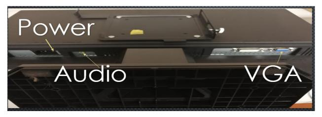
This is what you will be looking for, the blue and black cable up above. One end will run to the computer the other end will run to the monitor. It has two screws on the sides so make sure once you plug it in the right way that you secure it down with those screws. Once that is set in place the right way you should regain picture.
